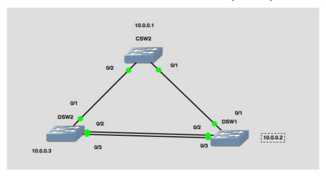
So for flexlinks, on DSW2, e 0/1 will become active. 0/2 will become backup (0/3 is down) Initially, ALL 3 switches are running R-PVST+
